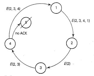
Figure 23.2 Election algorithm: RING.
