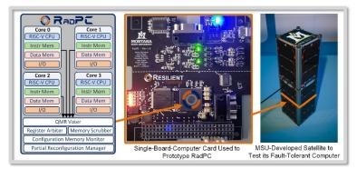
system output based on the majority of results from the cores in the event one core is faulted. In the event of a fault, the effected core is partially reconfigured to flush out any radiation-induced faults and then reintroduced into the system. RadPC has been flight tested on balloons (9x), sounding rockets (2x), the International Space Station (3x), and small satellites (2x). In 2023, it traveled to the surface of the moon for its harshest test yet.
