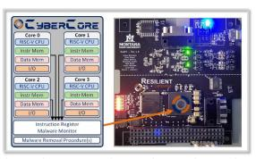
event of a malware attack, CyberCore will detect the malware as unknown instruction codes and flag the event. Once the computer detects an attack, the FPGA moves into a safe mode to continue processing. This research aims to provide an additional level of malware protection for critical computing applications.
