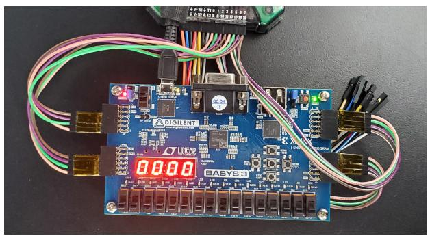
(a) Our prototype system, implemented and running on a Xilinx Artix-7 35T FPGA.
