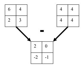
Now with the image on top of the approximation pyramid we can use the prediction residual images to rebuild the rest of the approximation tree. In this case we start with a single 4. Supersample it and add the  $2 \times 2$  prediction residual which gives:
