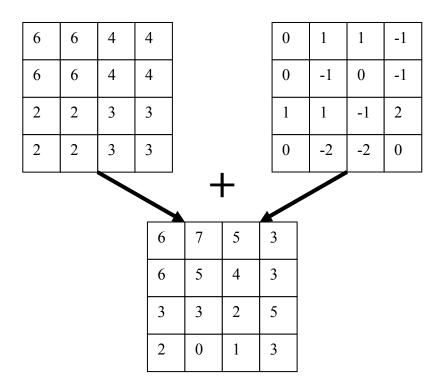
The gain here is that compression will be much better on the prediction residual images, because in areas of the image that have relatively constant intensity they will have values that are all at, or close to, zero. So by just saving the top image in a *P*-pyramid and the pyramid of residuals we can, with frequency-based encoding of the pixel values, achieve significant compression.
