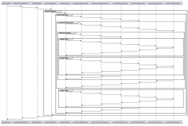
The UML diagram above shows the parsing of "var x = (2+2)\*5". It demonstrates the recursive nature of the CatScript parser, stemming from the natural recursive structure of grammars. The generated parse tree of "var x = (2+2)\*5" is as follows:
