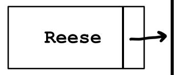
Blueprint for a single node in our data structure. Nodes have data, and a pointer to the next node
