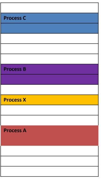
We split the process into smaller **pages**. Load pages into memory only when needed
