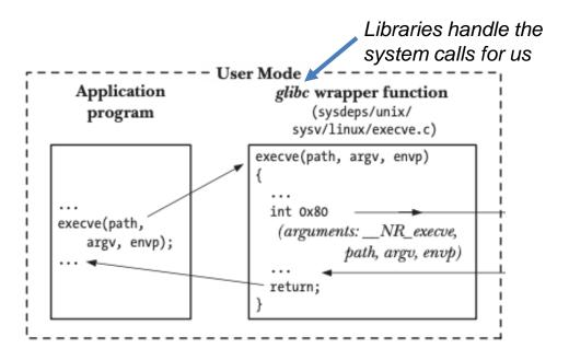
Applications evoke operating system defined functions, or system calls (syscalls), to access computing resources
