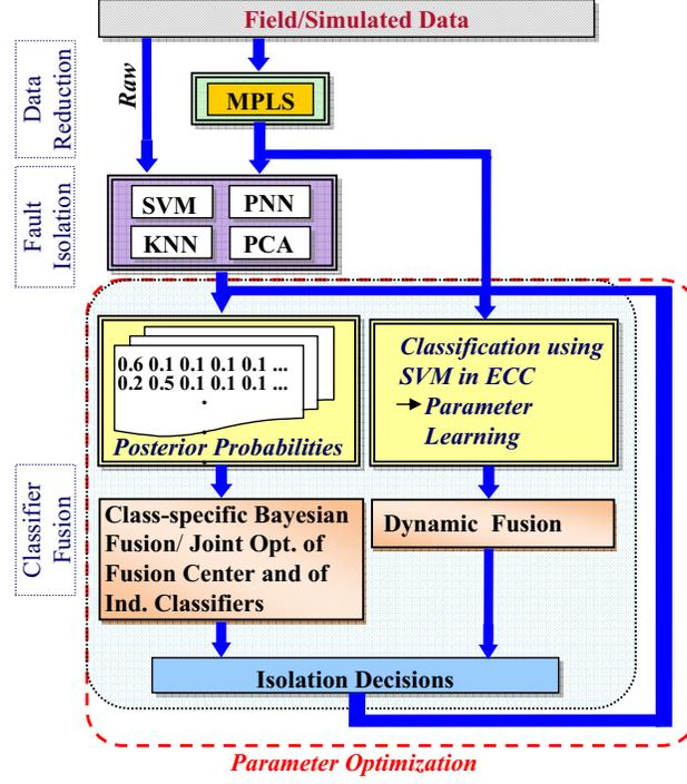
Fig. 1. Block diagram of proposed FDD fusion scheme.
