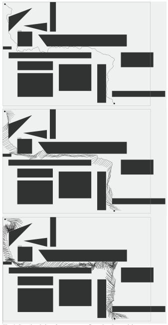
Fig. 6. Completed plans from a start configuration (lower right corner of each image) to a goal configuration (upper left corner of each image). From the top: a 2 dimensional point robot navigating the obstacles, a 3 dimensional rod robot navigating the obstacles, a 4 dimensional linked rod robot navigating the obstacles.
