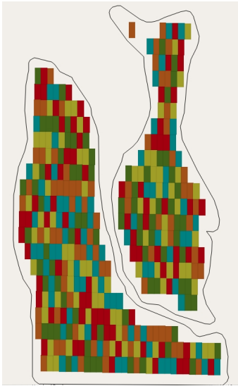
Fig. 1: Example prescription map for field “sec35mid.” Nitrogen rates 0, 20, 40, 80 and 120 pounds per acre correspond to red, orange, blue, light green, and dark green respectively.
