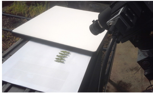
Fig. 3 A Resonon Pika L hyperspectral imager taking images of Kochia leaves in a controlled greenhouse setting.
