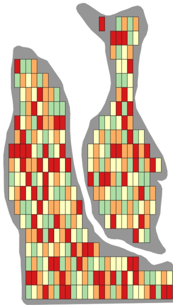
Figure 7.2: Example of a prescription map for experimental fertilizer application. Different colors represent different fertilizer rates.
