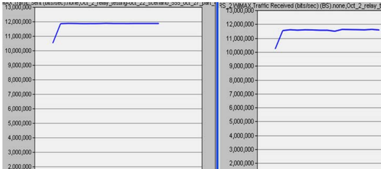
Fig. 5.19 – Traffic sent by SS vs traffic received by RS, scenario-8
