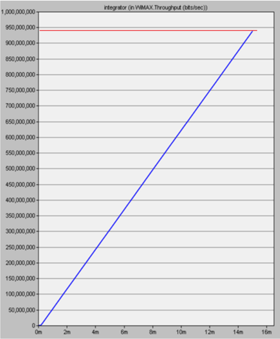
Fig. 6.13 – Total throughput (BS) for large scenario without implementing BFS+BHNB and IALU methods with directional antennas.
