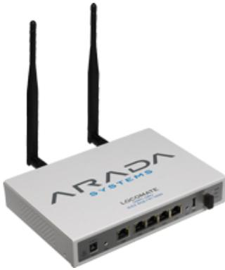
Fig. 1. The figure displays the OBU used in our experiment. More information can be found at <http://www.aradasystems.com/locomate-obu/>.
