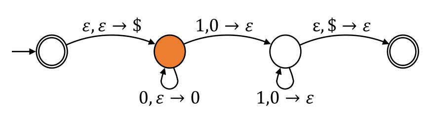
If 'a' is read from input and 'b' is on  $a, b \rightarrow c$ top of stack, pop 'b' and push 'c'.
