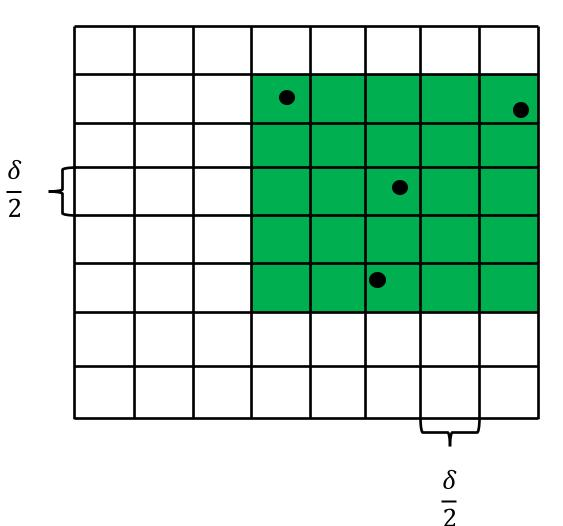
findClosestPair(on sequence P) Order points in random sequence  $\delta = d(p_1, p_2)$ Make map of cell size  $\delta/2$ for i = 1, 2,..., n Determine cell containing p<sub>i</sub> Lookup 25 cells surrounding p<sub>i</sub> Find dist to surrounding points if  $\exists p_i$  such that  $\delta' = d(p_i, p_i) < \delta$ Use  $p_i$  that make  $\delta'$  smallest
